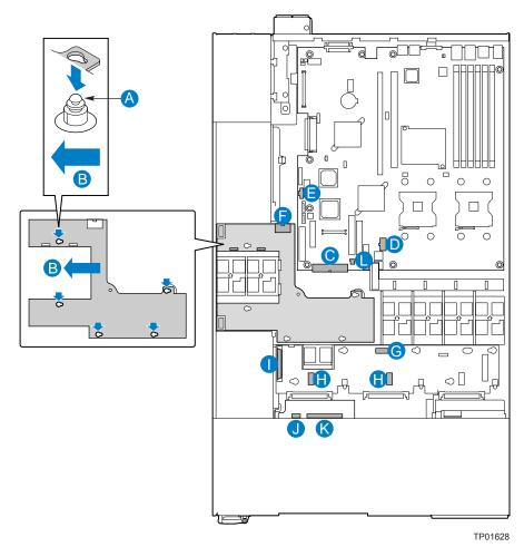
Figure 44. Installing the Power Distribution Board
